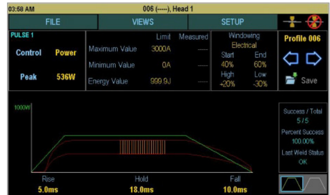
(Figure 2) Advanced part conditioning, single pulse, double pulses setups are easily viewed and adjusted.
