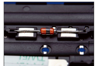
Component welding to leadframe
