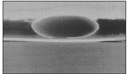
The adhesive normally consists of a mixture of thermoplastic and thermohardening (also known as thermoset- or duroplast-) glues, to get the best of both properties.
