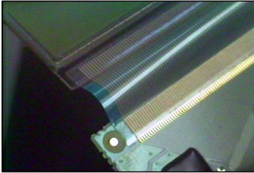
Laptop displays are a good example of ACF Bonding usage. A Chip On Foil technique is used here, one side of the foil is Hot Bar Reflow Soldered to a PCB and the other side is connected using ACF. When using the right production equipment, a extremely reliable joint can be made. Repair is possible, using new foils or using old foil from another display. This type of production is normally done on in-line production equipment.
