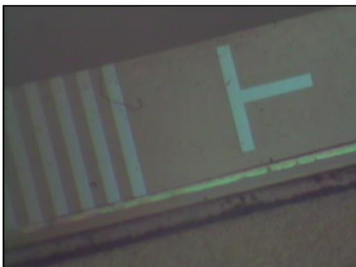
Looking through the flexconnector can be done only when a HSC is used. Another possibility is to use a "frame-freeze" option, where half of the image of the monitor is a frozen ITO image, taken before the flex was placed, and half the actual image, showing the flexconnector on top of the ITO.
