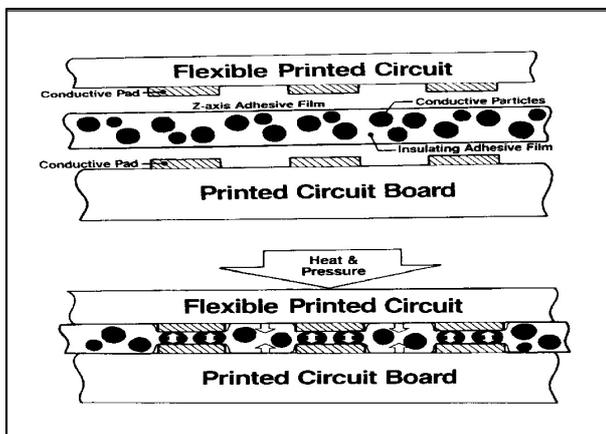
Before connection, an insulating adhesive film separates the conductive particles. When a heating element (normally called thermode) is pressing the top and bottom circuit board together, with the glue in between, the adhesive will flow, and conductive particles will be trapped, resulting in an electrical connection.
