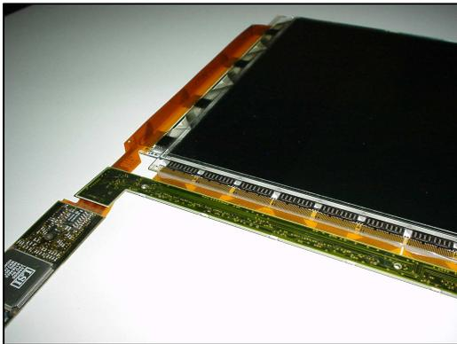
Automotive dashboards use more and more complex displays. This one is connected with Heat-Seal Bonding. Because of the large size, and the single connection, this type of application is normally done on a medium- to large-scale rotary table. The extreme environmental tests in the automotive industry do not form a problem any more with the newest Anisotropic Conductive Adhesives.
