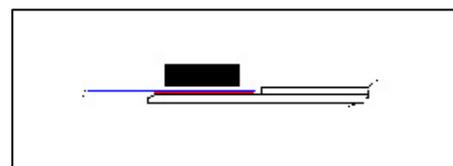
The next picture shows an example of how a HSC should not look like: there is no bevel and the foil bends downwards directly after the connection. The (matrix) glue that is pressed out should form a kind of meniscus and bend the HSC upwards. In this case the problem is caused by using a thermode that is too wide, or positioned too much near the
